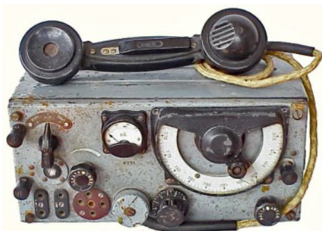
Photograph from an early version of the Russian A7 VHF FM transceiver taken at the Radio Amateur Museum in Budel. This FM transceiver operated in the frequency band 24-28MHz with a channel spacing of 100kHz. The RF output was 1.5-2W with a receiver sensitivity of 2µV. The working range with a rod aerial was up to 6km. A complete station weight 24.5kg.
